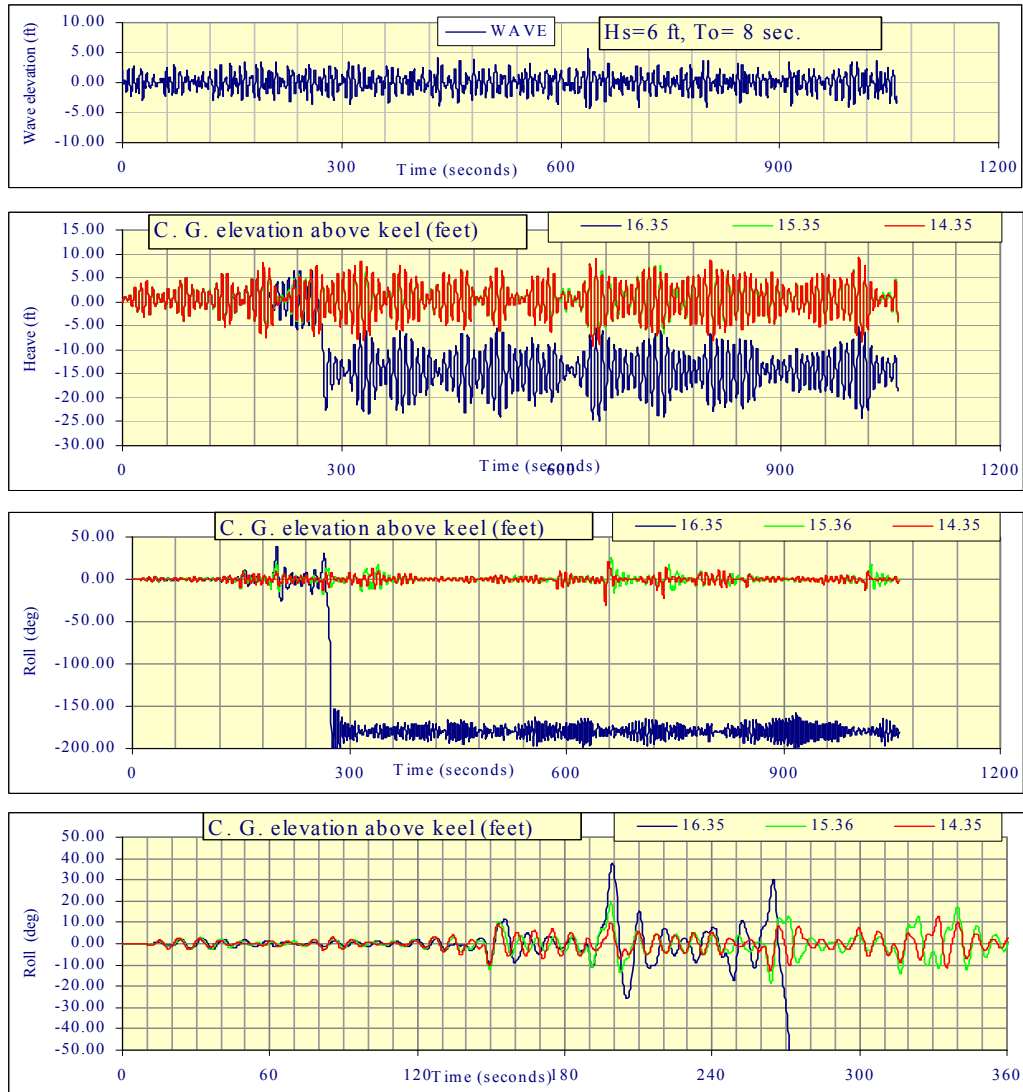
Figure 21. Sensitivity of the elevation of center of gravity to ship stability.
