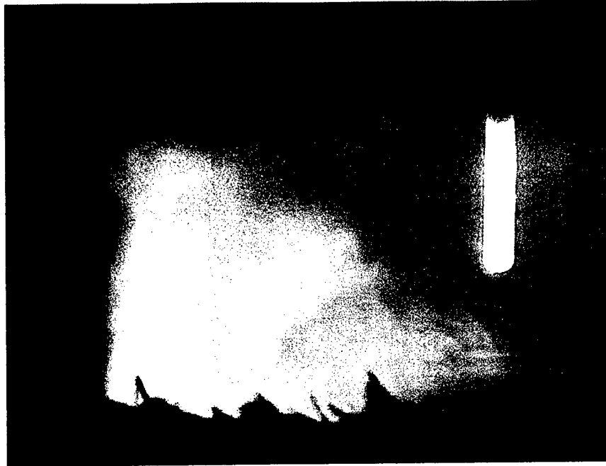
Figure 2.19: Reacting flow image at an equivalence ratio of 0.5.
