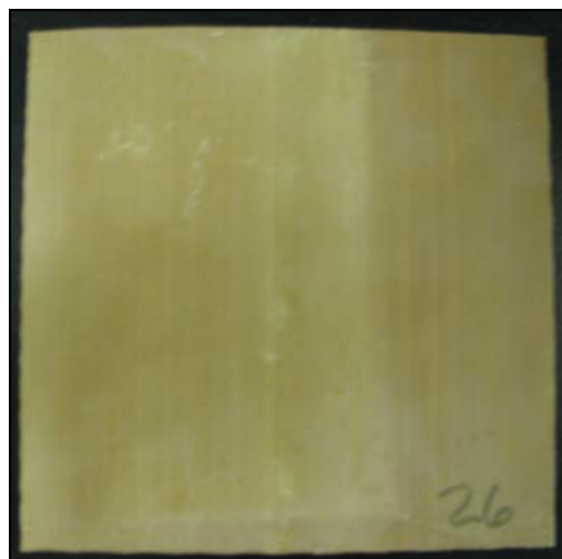
Figure 19. PVC 200-hour UV exposed specimen.
