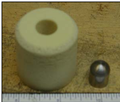
Figure 31. Tool steel hemispherical projectile with polyethylene foam sabot.
