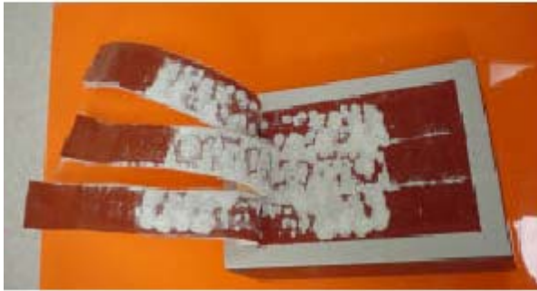
Figure 18. Peel without silane (avg peel = 6 lb/in). Figure 19. Normal peel (avg peel = 22lb/in).
