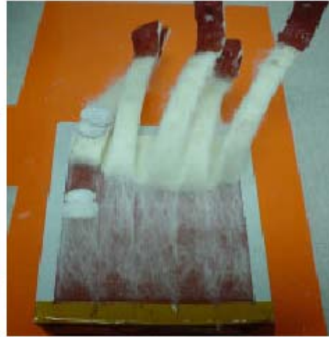
Figure 18. Peel without silane (avg peel = 6 lb/in). Figure 19. Normal peel (avg peel = 22lb/in).
