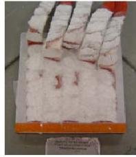
Figure 22. 3.61g RTV Applied
