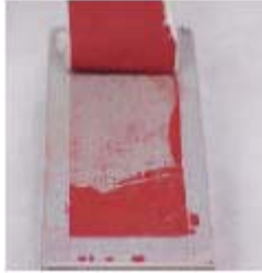
Figure 4. Similar OV-103 Subnominal SIP/IML Adhesive Bond.
