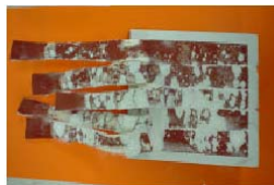
Figure 17. Peel without waterproofing (avg peel = 13.5 lb/in).
