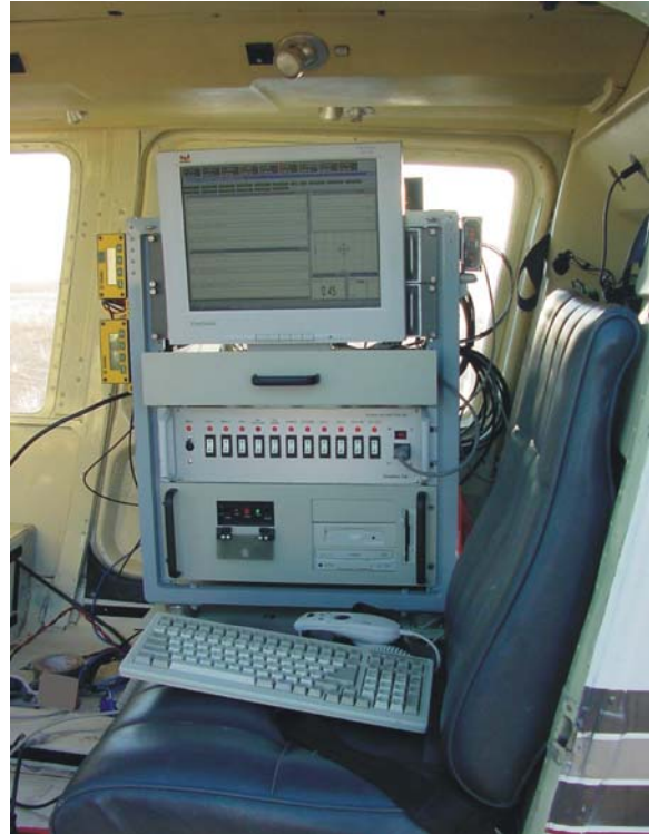
Figure 3 – The DAQ console is shown mounted in the rear starboard seat position. Note the Trimble Model MS-750 units mounted on the side of the rack.
