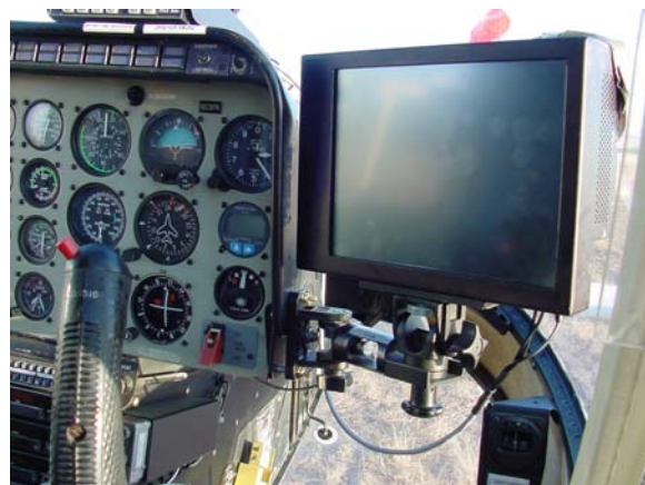
Figure 4 – Starboard side of the cockpit. The survey guidance display is shown mounted as it was used for the surveys.
