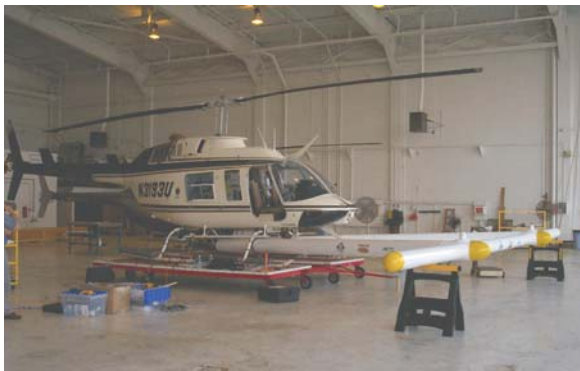
Figure 1 – MTADS Airborne Survey hardware is shown being installed on a Bell Long Ranger at the Helicopter Transport Services Hanger.
