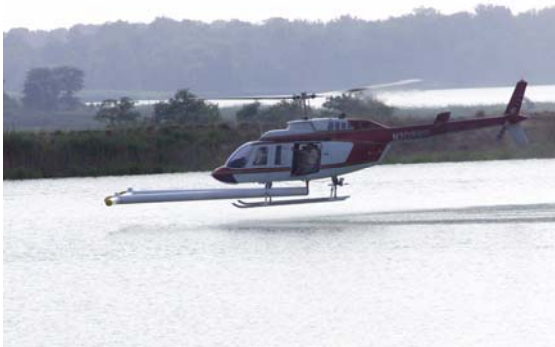
Figure 14 – MTADS survey over the larger pond.
