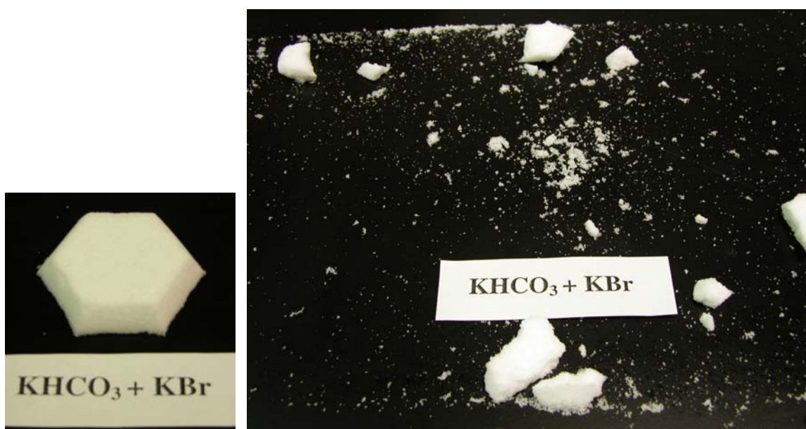
Figure 15. Adapted Anti-Cake Test II Results for the \text{KHCO}_3 + \text{KBr} as Additive
