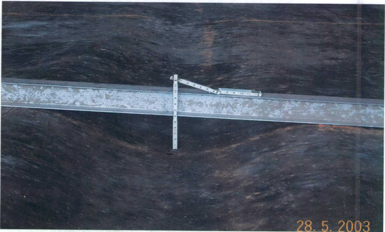
Photo 34. Measuring final rut depth on the Rapid Mat test (mat has been removed)
