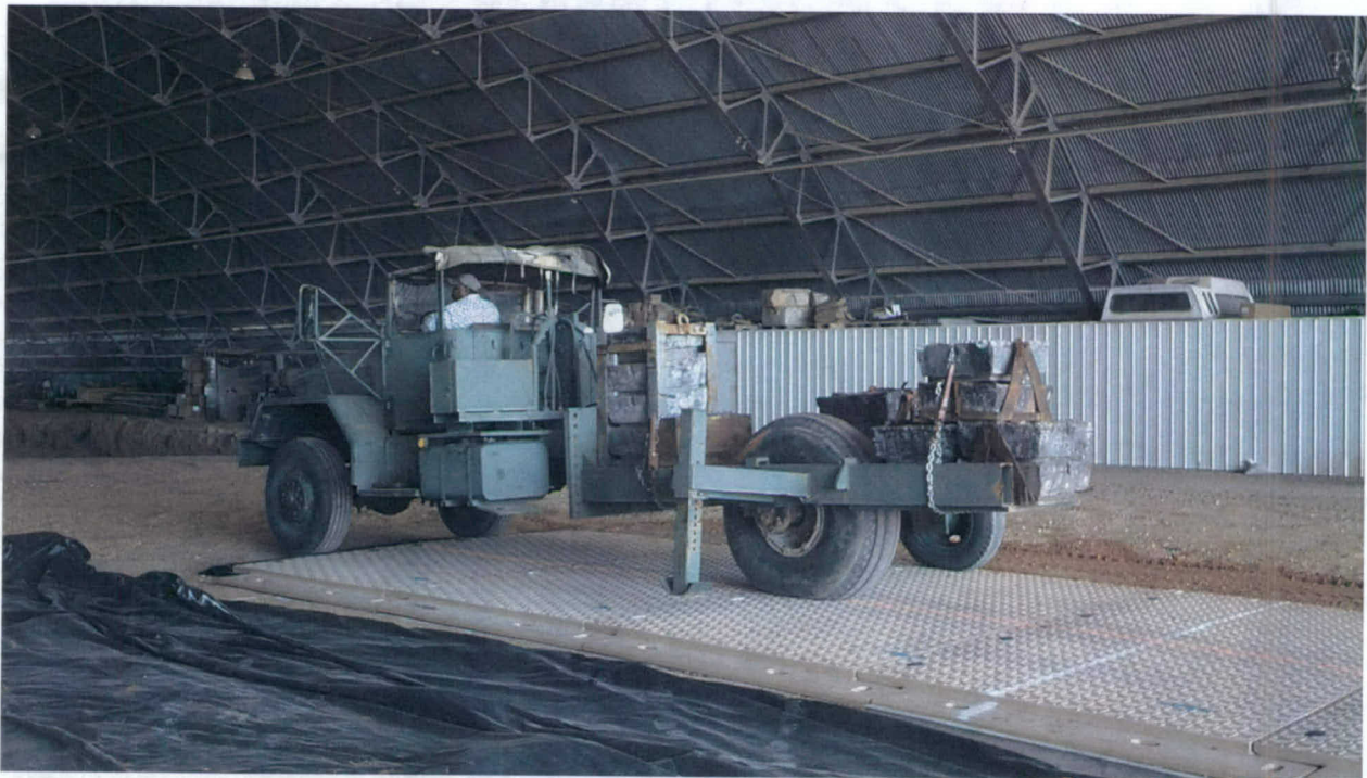
Photo 35. Loaded C-130 load cart performing traffic test on DURA-BASE matting
