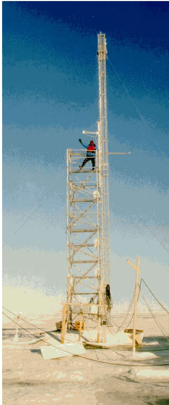
Figure 2. A tower used in the SHEBA field program served as a platform for measurements of temperature, humidity, surface wind vector, vertical heat flux, and vertical momentum flux at five different levels.
