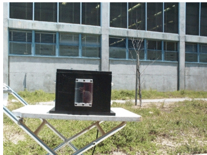
Figure 4. One of six light units from the TVE display. The single unit size is 18" (length) by 8" (height) by 10" (width). The unit was manufactured from non corrosive plastic and aluminum with a 105 watt halogen bulb.
