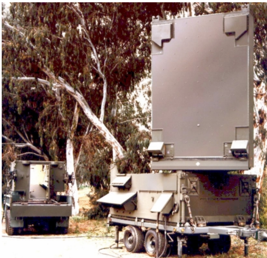
Figure 1 (above). AN/TPQ-37 Firefinder Counter Mortar/Counter Artillery Radar.
