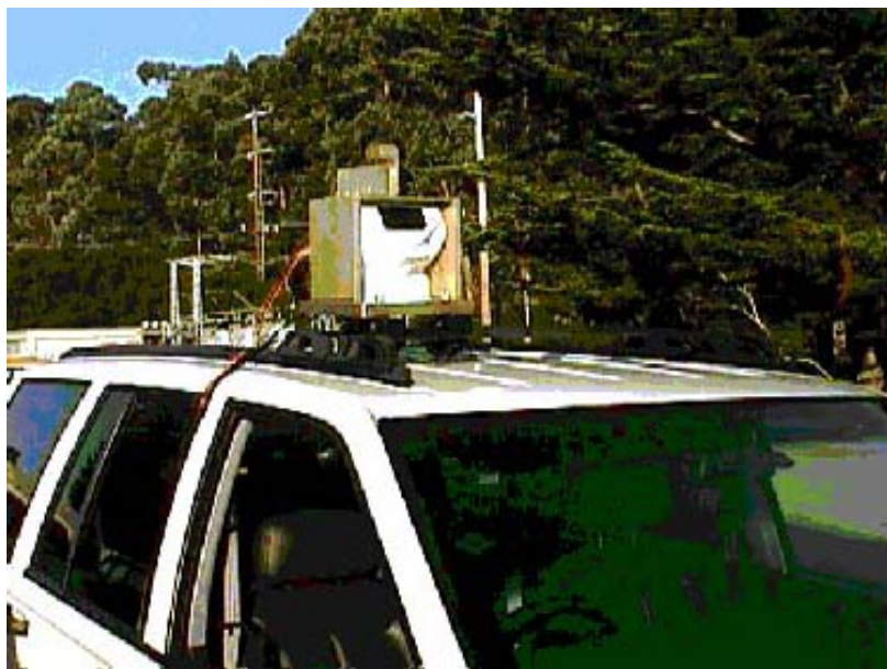
Image Sensor Fusion system mounted on a sport utility vehicle. The owner, LT James Elias, USN, is enrolled in the Test Pilot Student program within the Aeronautics Curriculum at the Naval Postgraduate School.
