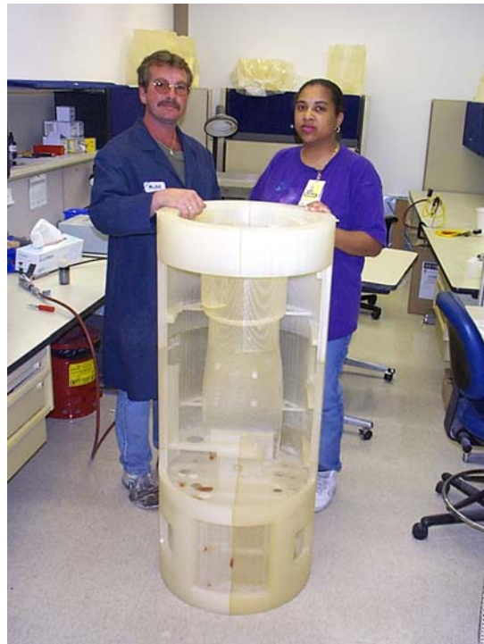
Figure 3. Example of a Large Part Produced by Stereolithography
