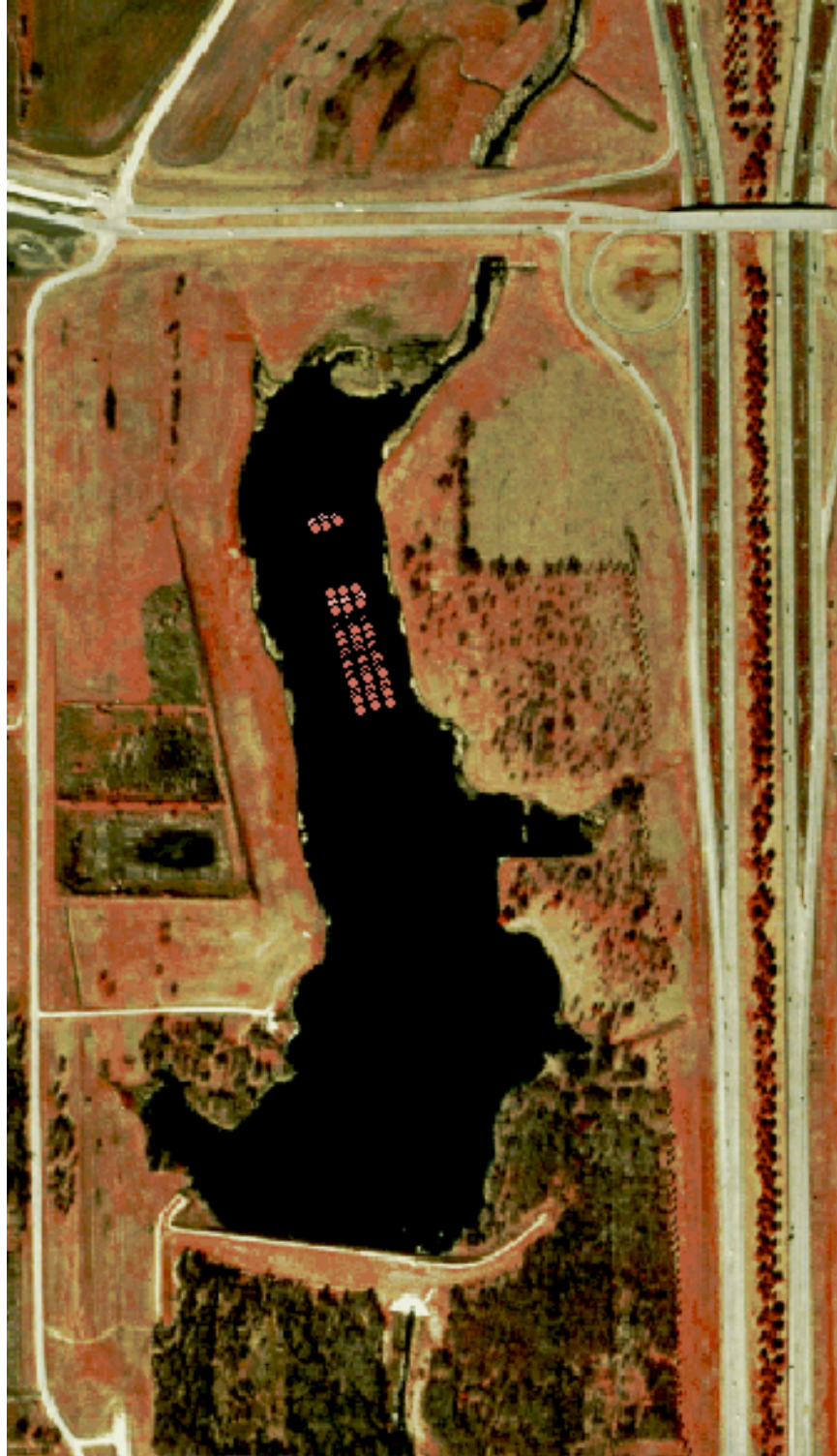
FIGURE A-10. THE DATA HAS BEEN TRANSFORMED BACK SO THAT THE POINTS ARE ACTUALLY IN THE CORRECT LOCATION. THE THREE SETS OF POINTS SHOW THE CENTER AND EDGES OF THE RADAR BEAM. THE COLOR SCHEME WAS CHANGED SO THAT DARKER REDS SHOW INCREASING ELEVATION.
