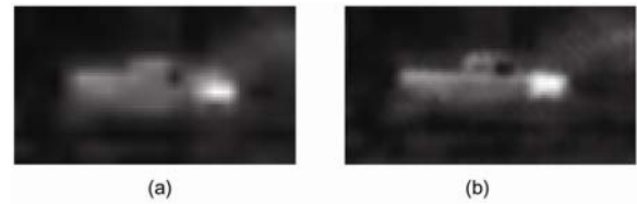
Fig. 7 FLIR images of a pickup truck. (a) Bilinear interpolated image. (b) Super-resolved image by the proposed algorithm.
