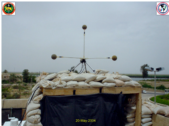
Fig. 1 – Tetrahedral Microphone Array
