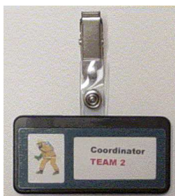
Figure 8. Locator tag that tracks humans/assets for the COORDINATORs system.
