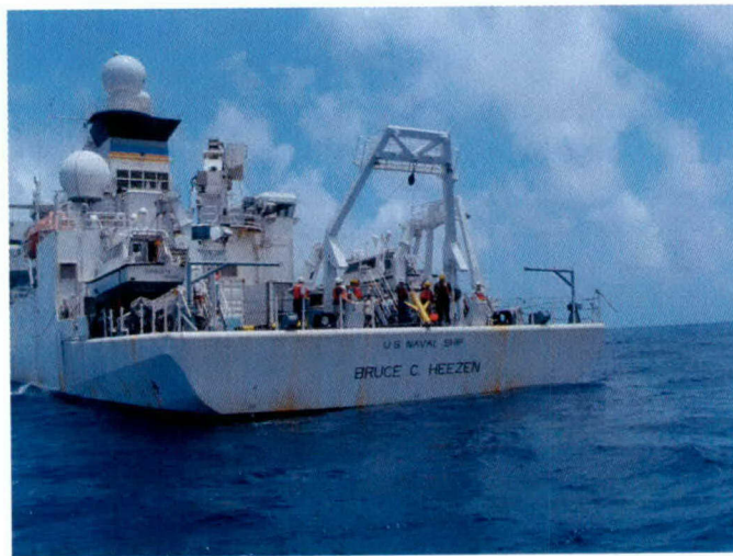
Figure 2: Glider deployment from the stern of the USNS Bruce Heezen in the western tropical Pacific. The vehicle was lowered to the water using a winch and then set free using a quick release on the hoisting line.
