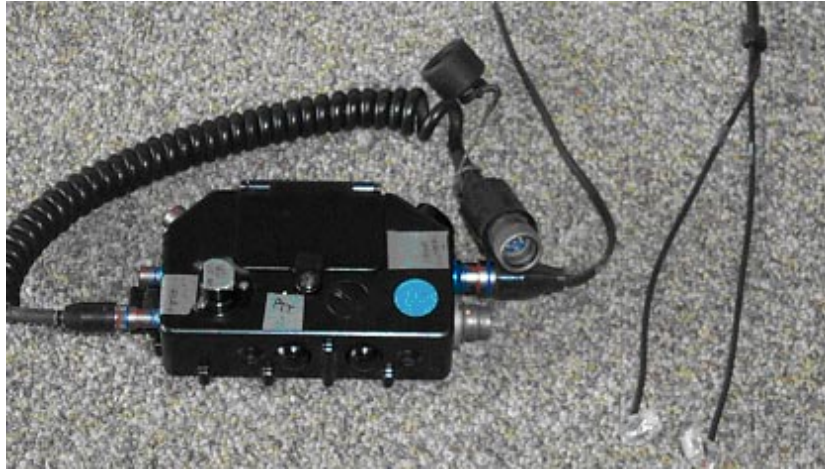
Figure 3. Components of TAC system: interface box with push-to-talk buttons, volume control, earplugs (disposable foam tips not shown).
