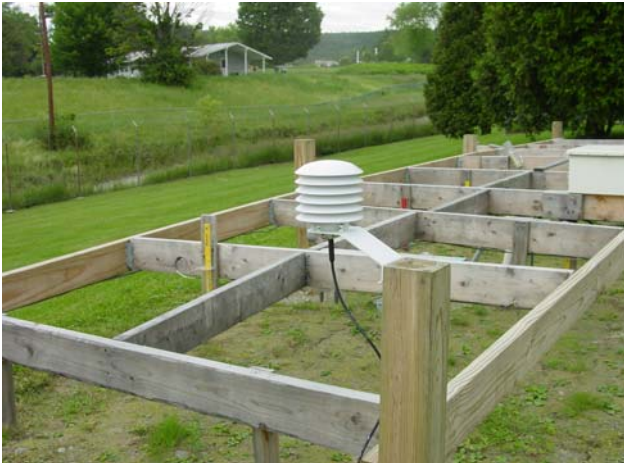
Figure 2. Test frame for frost-jacking experiment.
