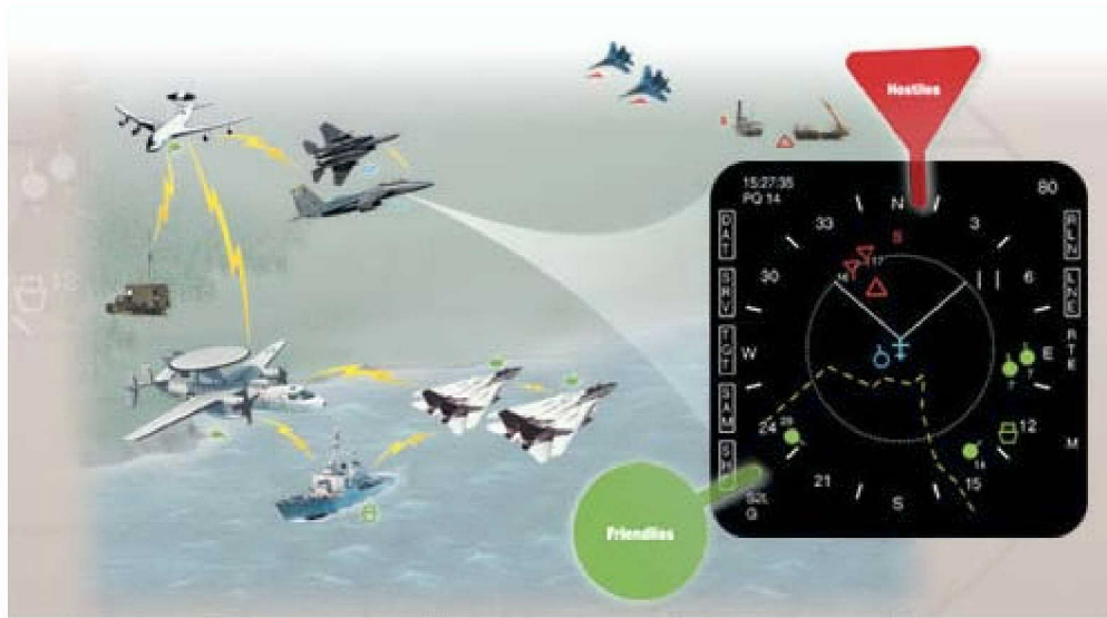
Figure 37. Link 16 provides highly accurate position data and identification of friend or foe (IFF). 78
