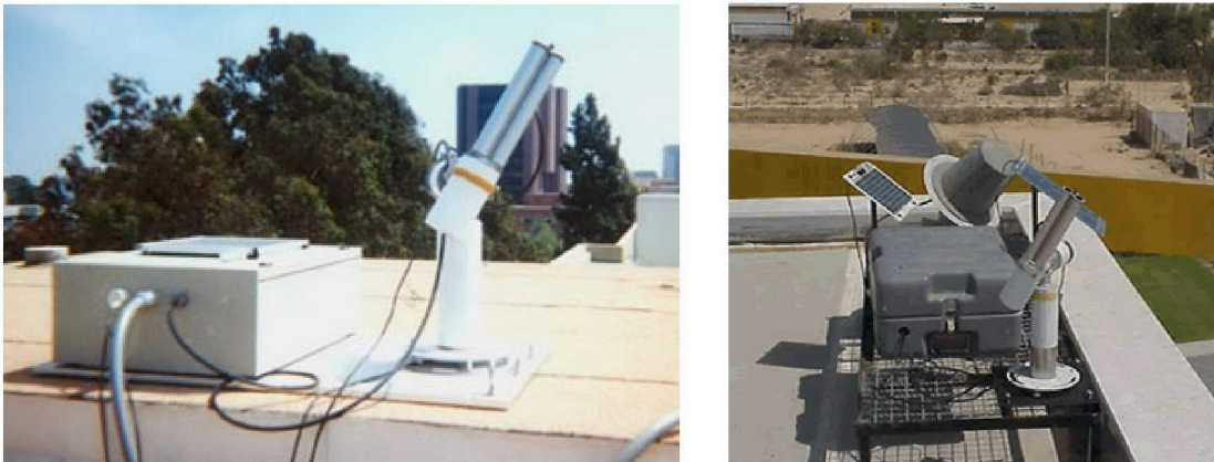
Figure 6. CIMEL Spectral Radiometer (from Holbren, 2004)
