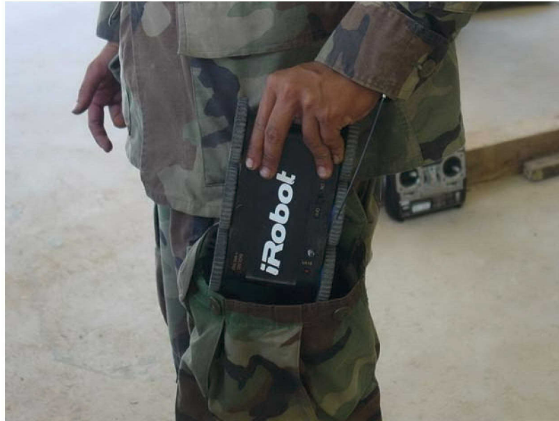
Figure 11. Phase I ThrowBot was designed to fit into standard thigh pocket.
