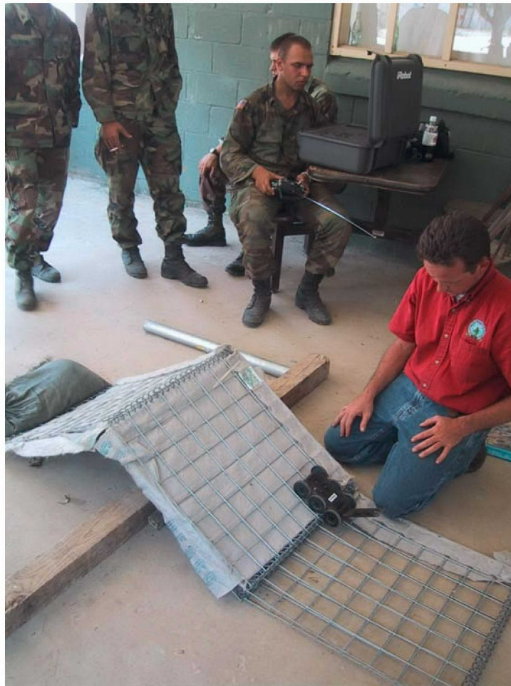
Figure 10: Six-wheel ThrowBot climbing over open grate.
