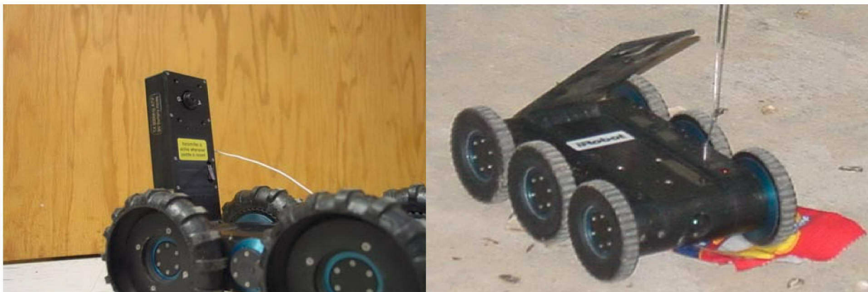
Figure 13. Cameras are mounted on the paddle (left) and in the nose (right) of the Four- and Six-Wheeled ThrowBots.
