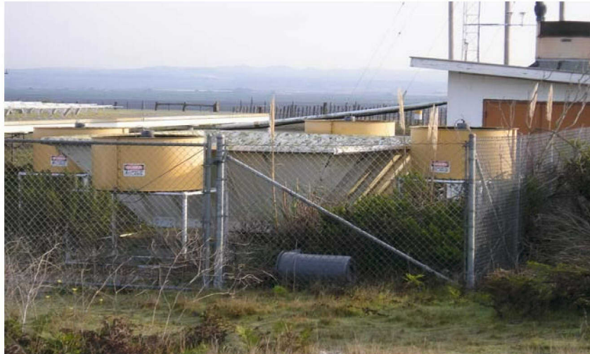
Figure 4. NPS 915 MHz Profiler/RASS system at MAML.
