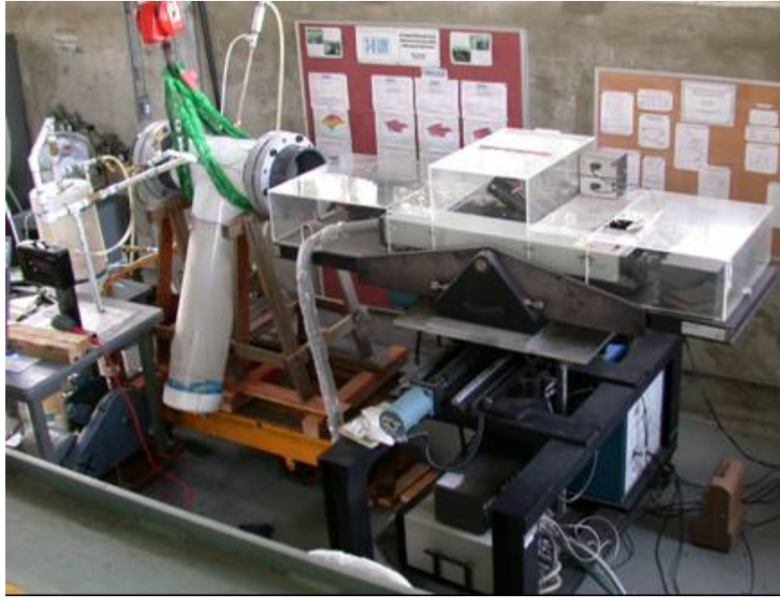
Figure 47. Traversing LDV system set on the vacuum test chamber
