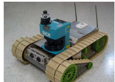
Figure 2. JPL's PackBot equipped with TMR-era stereo and laser collision-avoidance sensors.
