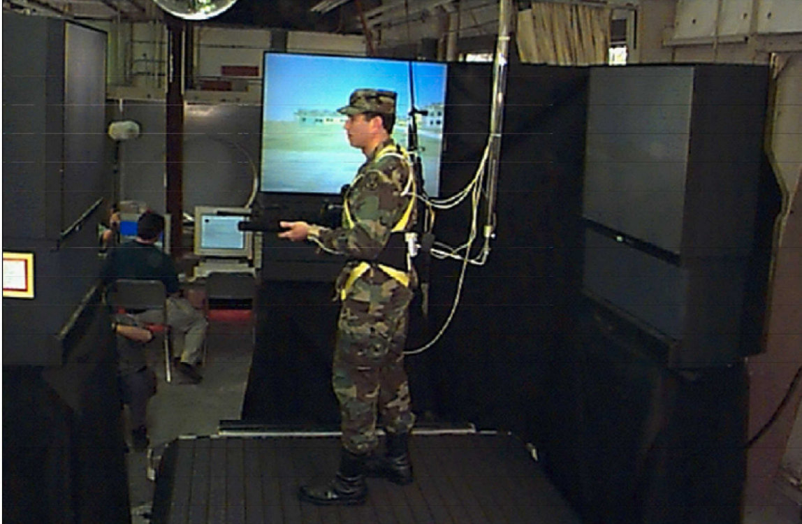
Figure 10. Omni-directional Treadmill (ODT) Photo courtesy of Darken, R. Naval Postgraduate School, Monterey, CA.
