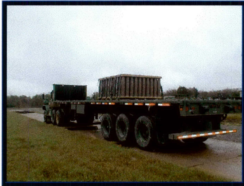
Photo 15. Hazard Course Testing of the M872 A4 Semi Trailer with the 155MM Separate Loading Projectiles
