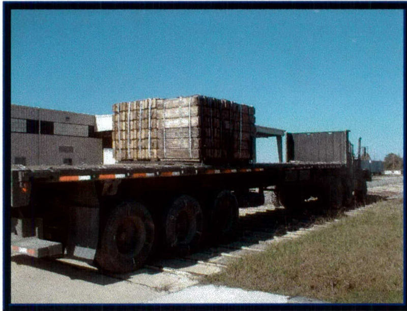
Photo 19. Washboard Course Testing of the M872 A4 Semi Trailer with the C445 Load
