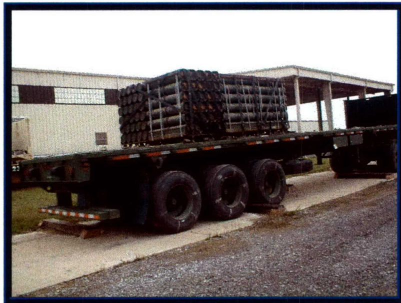
Photo11. Hazard Course Testing of the M872 A4 Semi Trailer with the 120MM Tank Ammunition
