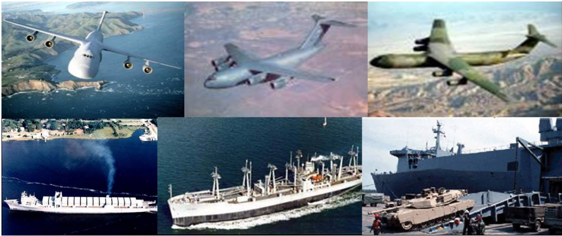
Figure 3. Clockwise from upper left C-5, C-17, C-141, RORO ship offloading a tank, Breakbulk ship (Cape Gibson), and Light Aboard Ship (LASH, similar to a civilian container vessel).
