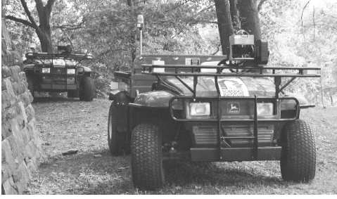
Figure 7: The autonomous E-Gator platform.
