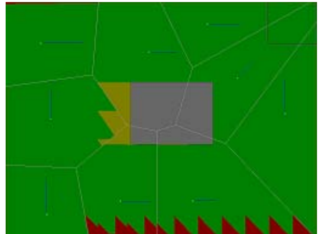
Figure 6: Color map using three different colors to represent cost groups (screen capture from PTMS software). A large rectangular obstacle is in the middle of the playing field. A majority of the trajectories will terminate at the goal (upper right hand corner). Others will stagnate at the obstacle or leave the playing field (red saw-tooth structure at the bottom).
