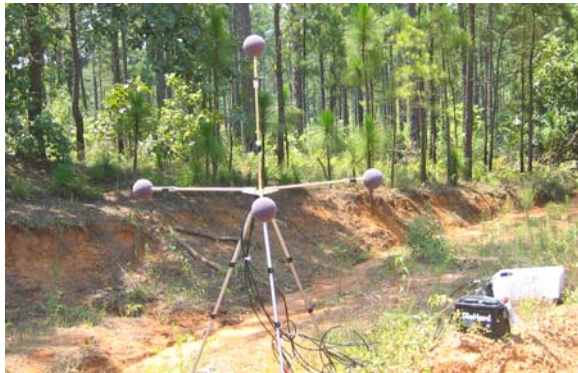
Figure 12: 1-m tetrahedral UGS acoustic array for transient detection, with battery, tripod and processor.
