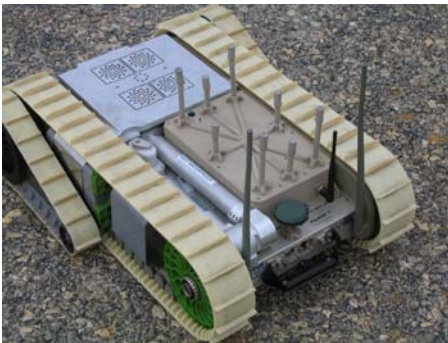
Figure 10: PackBot with 8-mic array, extensible imaging head, GPS and communications antennae.
