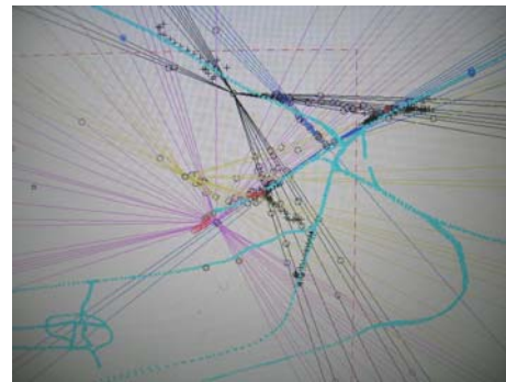
Figure 16: Screen dump of UGS LOBs and detections from other vehicle-mounted arrays demonstrating the complexity of the tracker's job. Blue represents roads.
