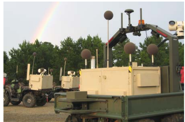
Figure 13: Acoustic sensors with windscreens shown on the RSV (right) and two ATV's (left).
