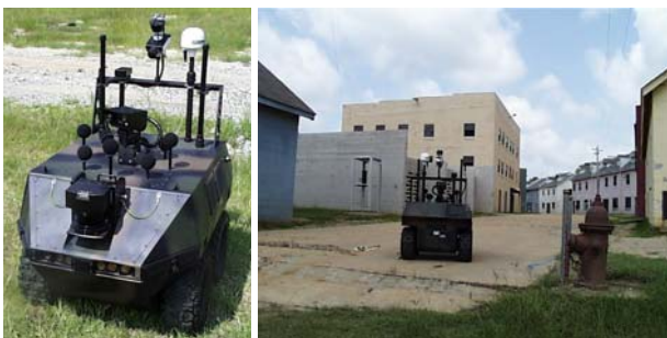
Figure 1: ATRV-II robot acoustically cues cameras mounted on a pan/tilt when sniper fires from roof.
