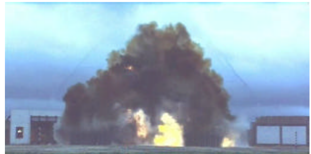
Fig. 9. Wall retrofits using trowel-on elastomers are subjected to full scale blast effects in experiments at Eglin AFB.
