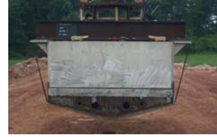
Figure 6. Photograph of the Phase II kit attached to structure and VIMF guide rail.
