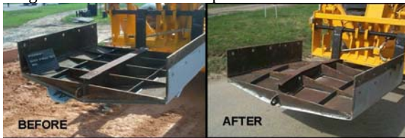
Figure 4. Before and after experiment photographs of stiff steel wedge structure
