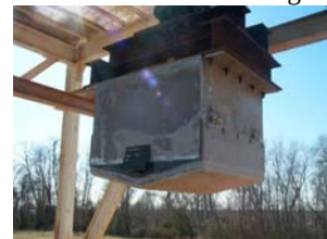
Figure 2. Photograph of quarter scale aluminum hull structure and wedge kit made of steel, concrete, and S2 composite.
