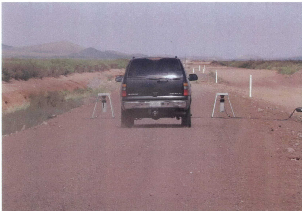
Photo 42. Light dust produced by vehicle traveling Section 14, Dust Fyghter®
