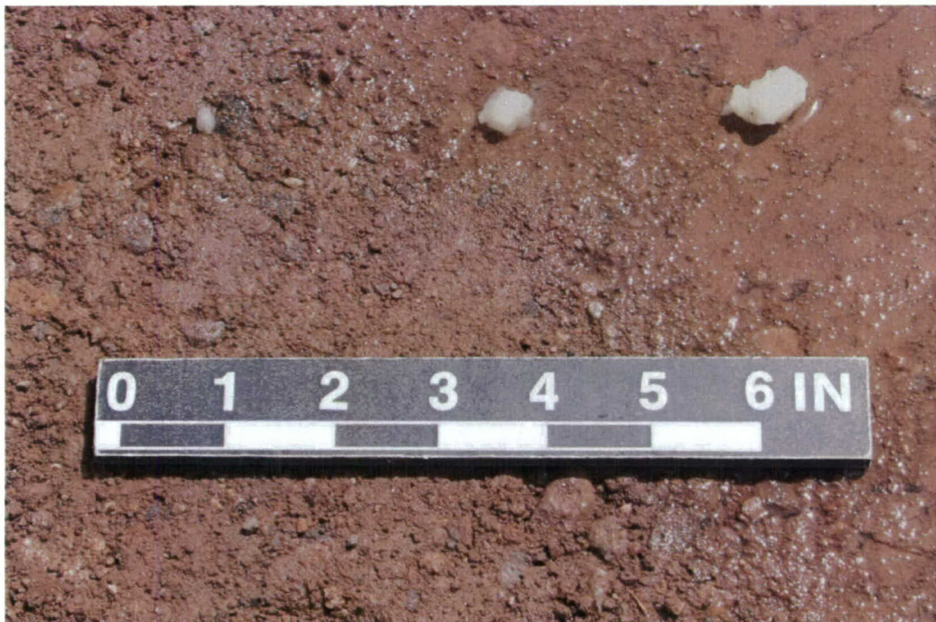
Photo 32. Balls of undissolved Hydrostik® sprayed from hydroseeder
