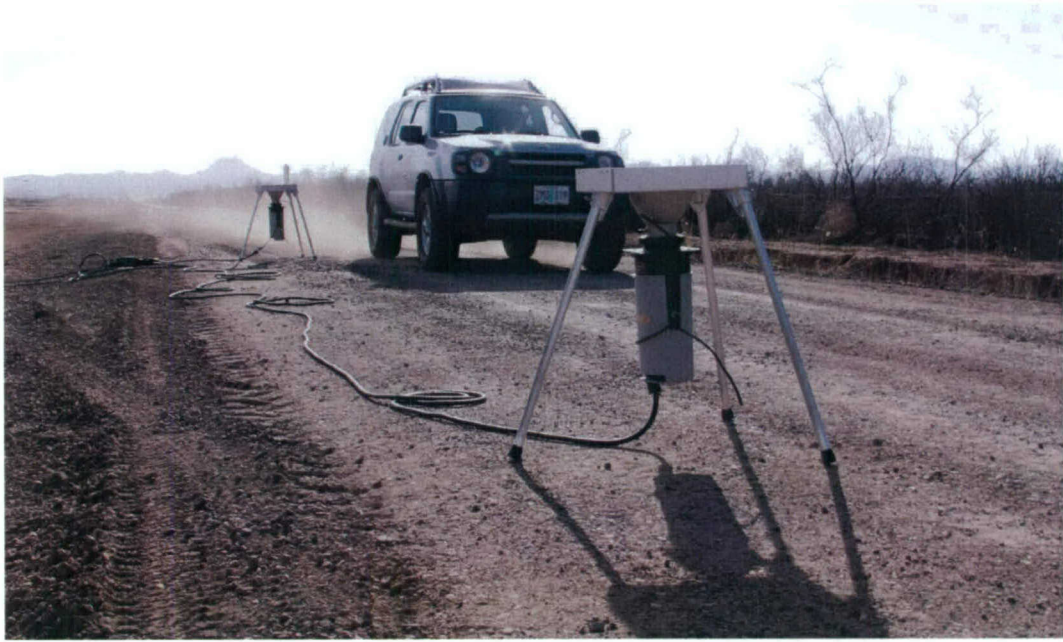
Photo 23. Use of SUV to apply traffic during dust collection
