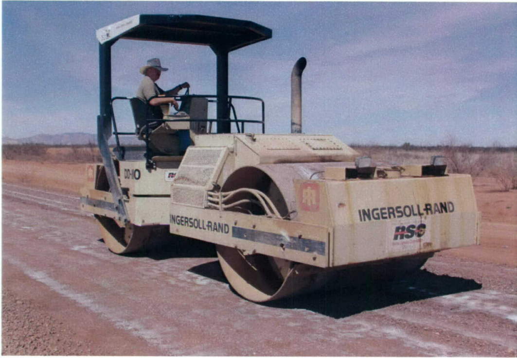
Photo 9. Ingersoll-Rand 12-ton vibratory compactor
