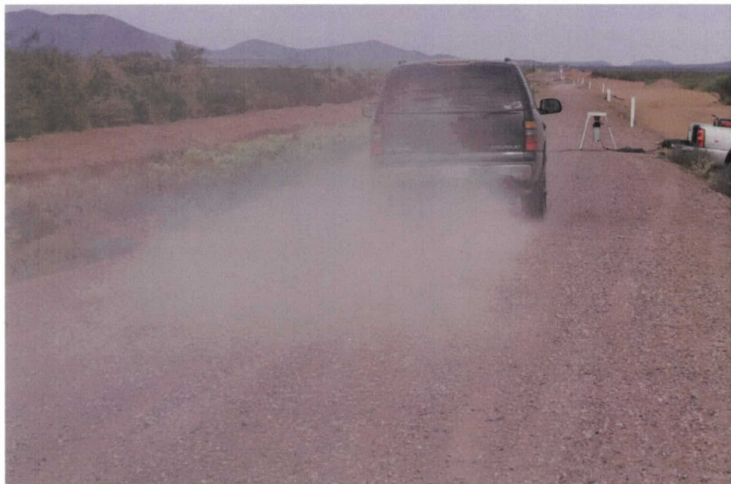
Photo 40. Dust collection on Section 12, Blue Goo®
