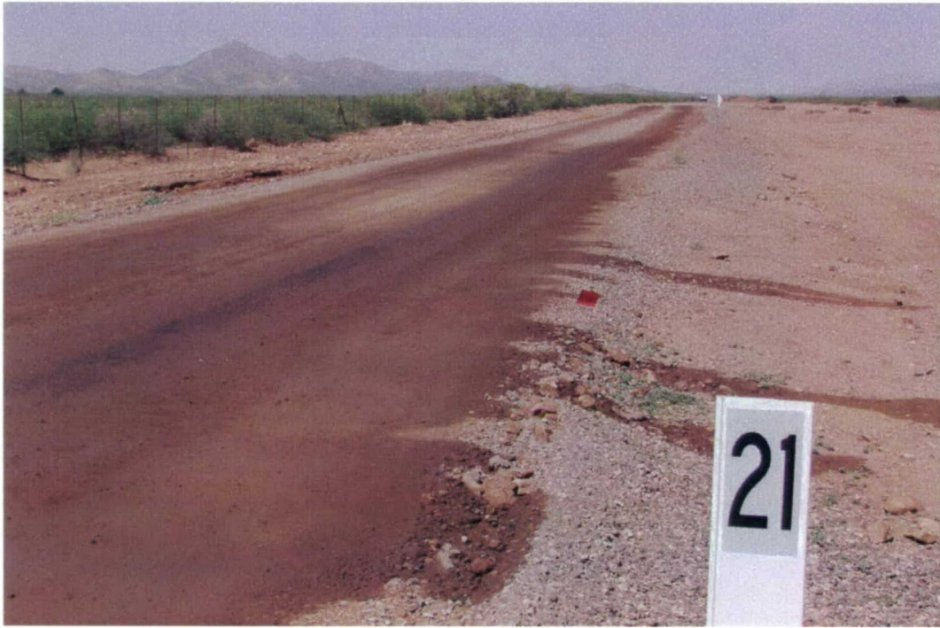
Photo 37. Uneven product distribution on Section 21 after 30 days
