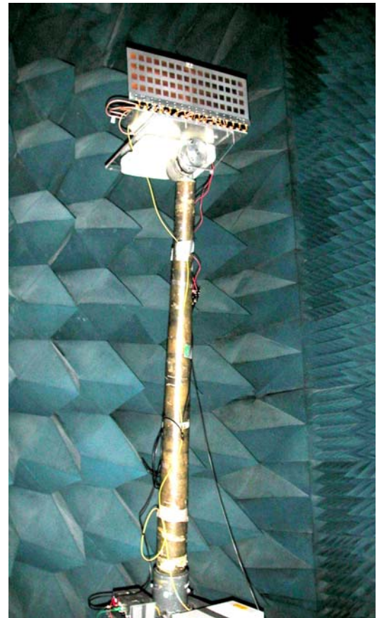
Figure 7. The Photonic phased array antenna system in the microwave test chamber.
