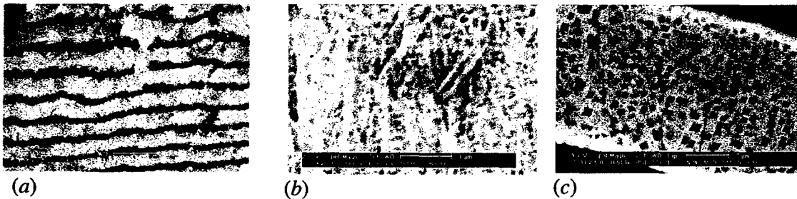
Figure 3: Cross sectional scanning electron microscope images of \gamma -Ni(Al)/ \gamma' -Ni 3 Al multilayers for (a) \Lambda = 300\text{nm} , f_{\gamma\text{-Ni(Al)}} = 0.6 after 1073K/10 hr, (b) \Lambda = 50\text{nm} , f_{\gamma\text{-Ni(Al)}} = 0.5 after 1273K/0.5 hr, and (c) \Lambda = 240\text{nm} , f_{\gamma\text{-Ni(Al)}} = 0.5 after 1373K/20 hr.
