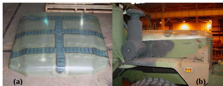
Figure 7: Photographs of (a) the unpainted composite hood and (b) the hood affixed on an M35-A3 truck. The blue stripes are PVC foam stiffeners that are fabricated into the part.
