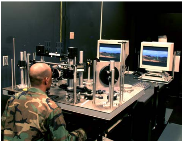
Fig. 2 The in-device optical setup for optometric tests and experimental misalignment tasks. It simulates a see-through, daytime, partial-overlap biocular HMD
