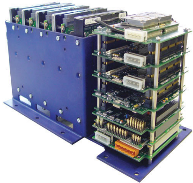
Figure 11 – HPEC application using Nallatech FPGA COTS products [9]
