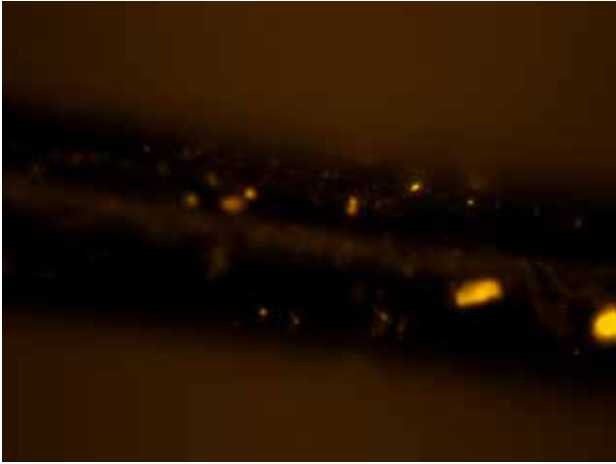
Figure 6. Fluorescence image of CdSe-ZnS/CdS/CdSe-ZnS/CdS-coated Au wire with a collection window of 585 \pm 40 nm.
