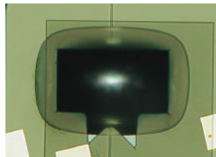
Figure 10 - Waveguide facet and detector polymer well
