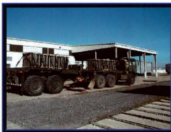
Photo 8. Hazard Course Testing of the FMTV 5-Ton Truck and Trailer with the 155MM Separate Loading Projectiles
