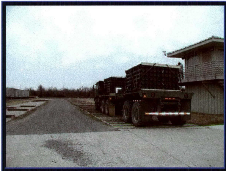
Photo 18. Washboard Course Testing of the FMTV 5-Ton Truck and 5-Ton Trailer with 120MM Tank Ammunition
