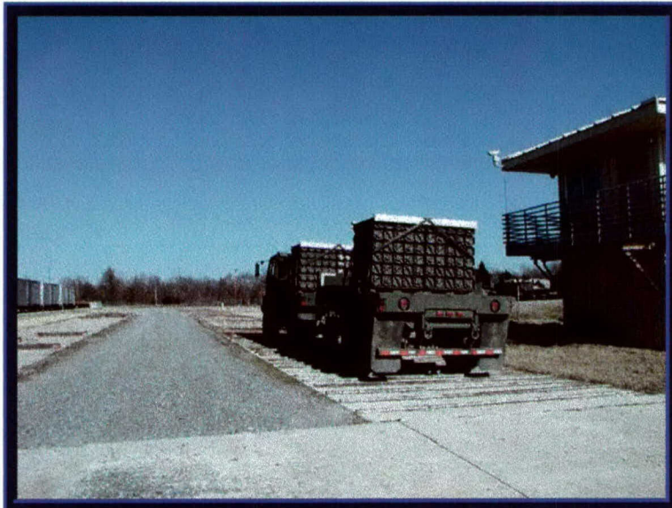
Photo 16. Washboard Course Testing of the FMTV 2.5-Ton Truck and Trailer with 120MM Tank Ammunition
