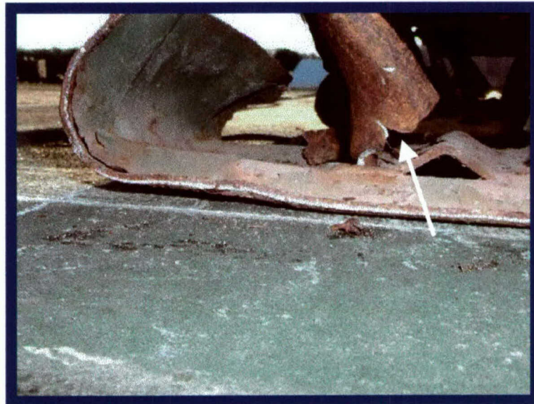
Photo 13. Damage to the Pallet from the Strap
