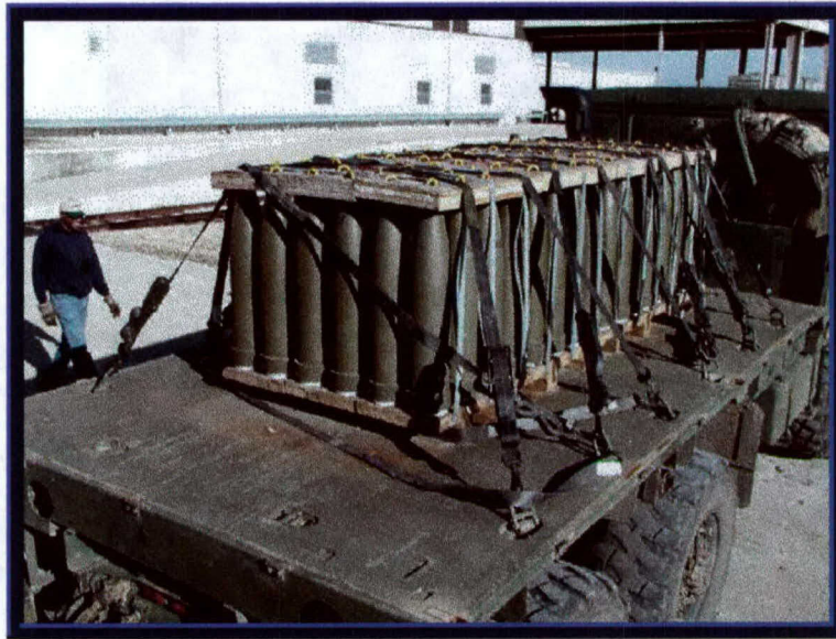
Photo 10. Disengaged Cross Strap at Aft End on the Truck
