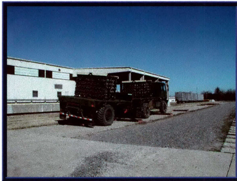
Photo 15. Hazard Course Testing of the FMTV 2.5 –Ton Truck and 2.5-Ton Trailer with 120MM Tank Ammunition
