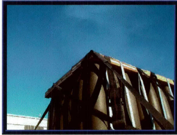
Photo 9. Slipping Cross Strap at Aft End on the Truck
