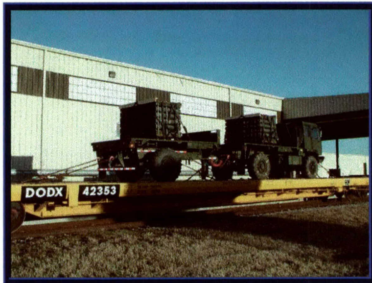
Photo 14. Rail Impact Testing of the FMTV 2.5-Ton Truck and Trailer with 120MM Tank Ammunition (Prior to Testing)
