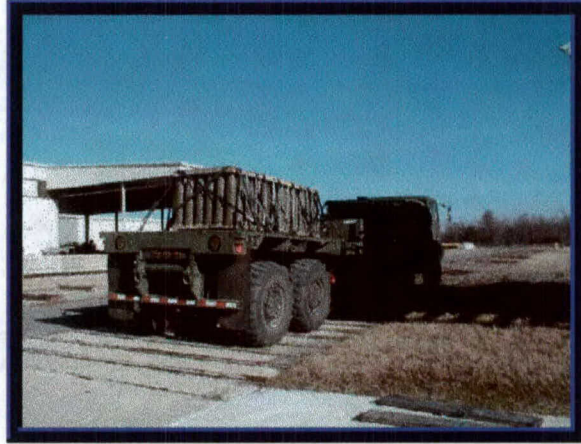
Photo 11. Washboard Course Testing of the FMTV 5-Ton Truck and Trailer with the 155MM Separate Loading Projectiles
