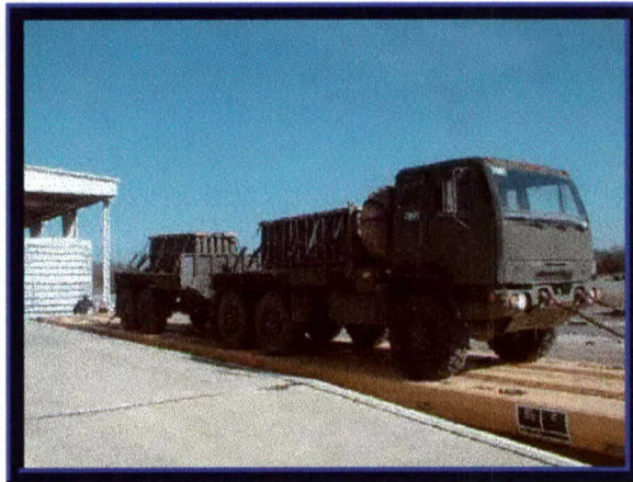
Photo 5. Rail Impact Testing of the FMTV 5-Ton Truck and Trailer with 155MM Separate Loading Projectiles (Prior to Testing)
