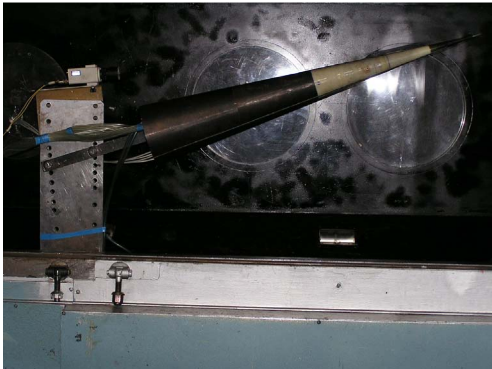
Fig. 1.18. View of turbulisers and smoke hole
