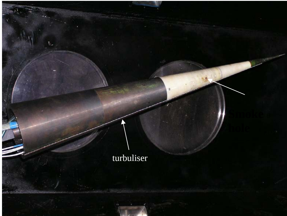
Fig. 1.18. View of turbulisers and smoke hole
