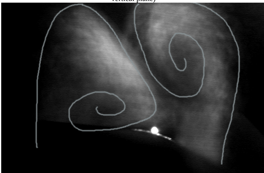
Fig. 1.6. Laser knife flow visualization, frame 92. (gray lines show streamline projections on the vertical plane)
