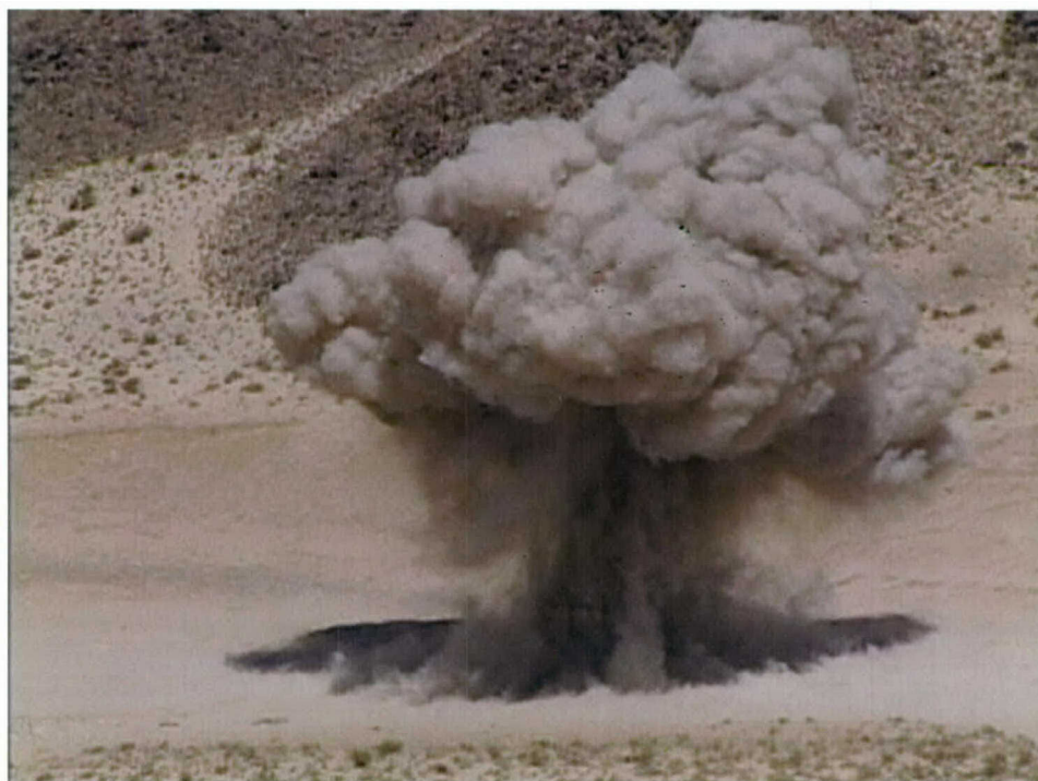
FIGURE 7. Still Photo Taken From High-Speed Motion Picture of an Open Detonation Event at China Lake. The highly visible plume is dirt from the initial crater and entrained dirt.
