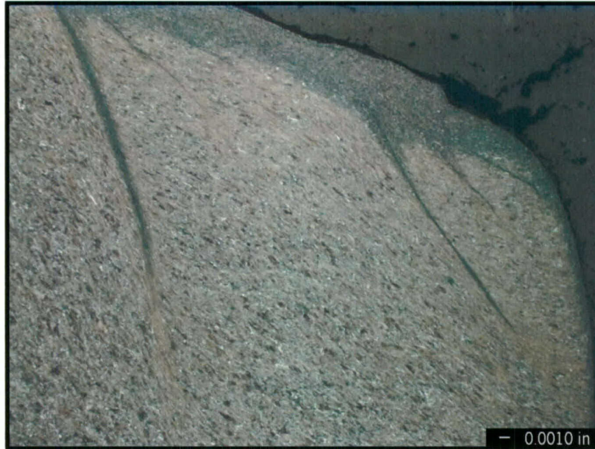
FIGURE B.6. Shear Bands Noted on the Edge of Steel Sample 3. Note the deformed grains adjacent to these bands. Etchant: 5% Picral. Original mag. 100x.
