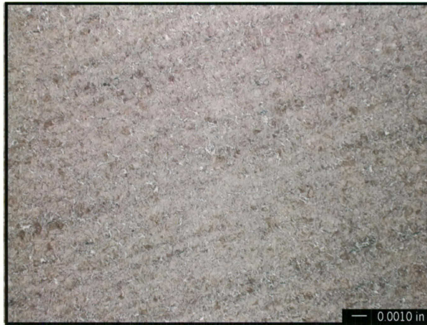
FIGURE B.10. Flow Lines Noted Emanating from the Interior Surface of the Projectile Body, the Result of Prior Forging. Original mag. 200x.
