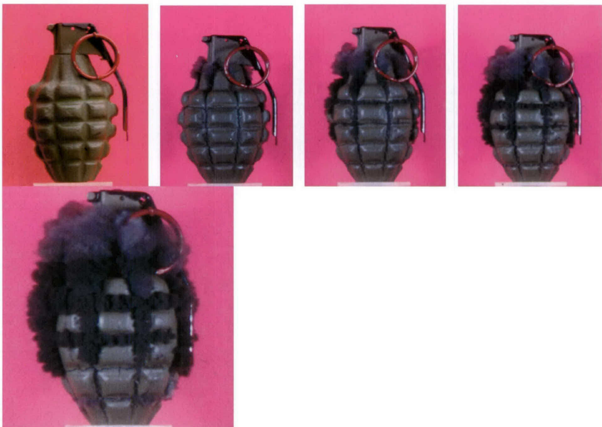
FIGURE 13. Still Photos Taken From Ultra High-Speed Motion (ca. one million pictures per second) Pictures of Detonation of a Grenade.
