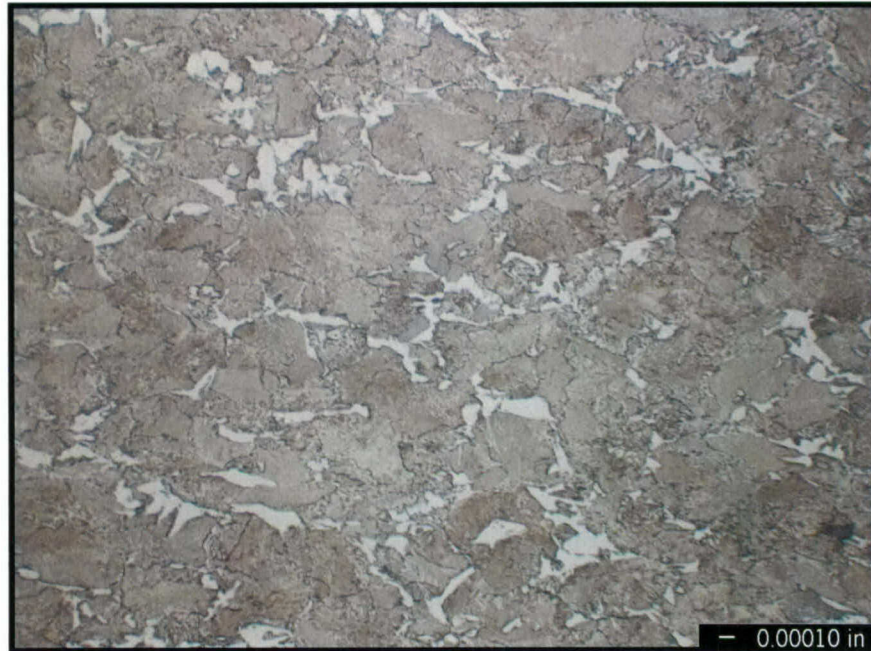
FIGURE B.4. Microstructure of Pearlite with Ferrite Islands Along the Grain Boundaries, Which was Predominant on Each of the Steel Samples Examined. This structure was most likely formed during original processing. Original mag. 1000x.
