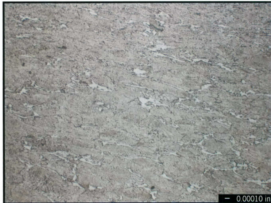
FIGURE B.5. Microstructure of Elongated Pearlite with Ferrite Observed Mainly Closest to the Exterior Surface of the Projectile Body. Compare to Figure B.15. This structure was most likely formed as a result of the energy produced during detonation. Original mag. 1000x.
