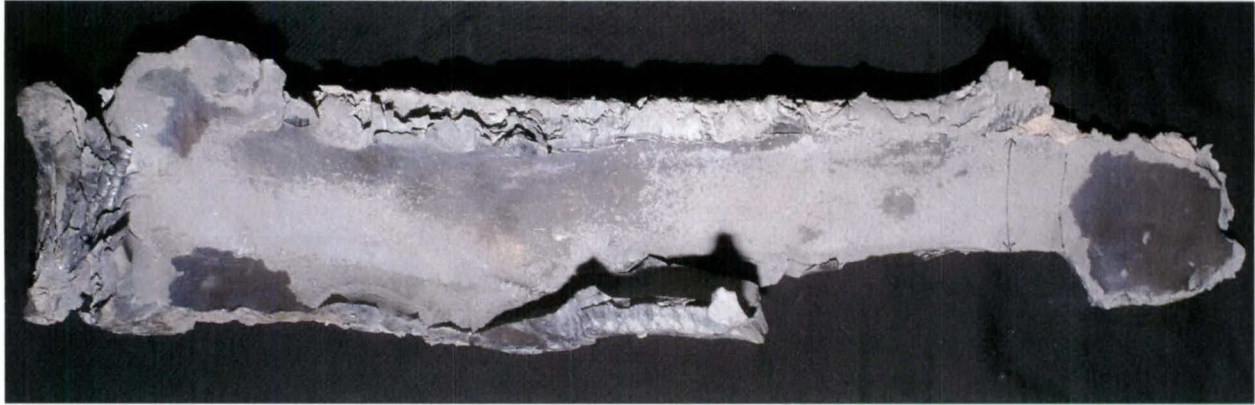
FIGURE B.1. Original Fragment from the Exploded M107 Ordnance. Reduced ~67%.
