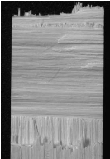
Figure 28. Tensile Fracture Surface of N610/Alumina at 23°C
