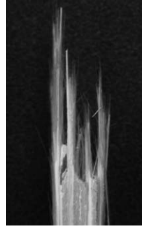
Figure 43. Tensile Fracture Surface of N610/Mon/Alumina at 1200°C (Side)
