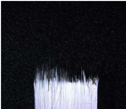
Figure 69. Creep Fracture Surface of N610/Mon/Alumina at 1100°C, 40 MPa
