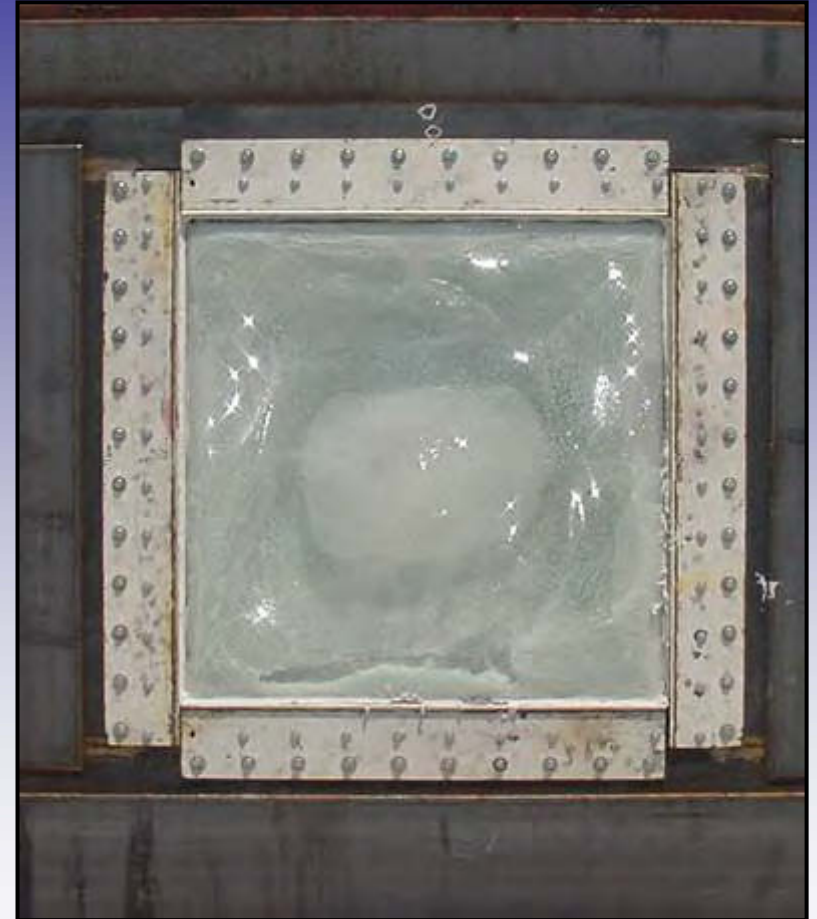
Posttest Photo of Blast Side
