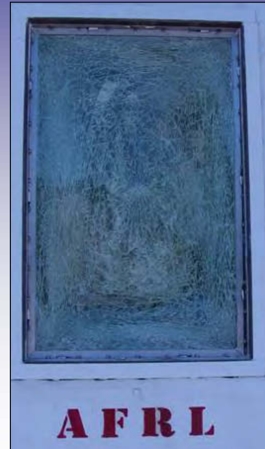
0.270" PVB Clamped Tail SUCCESSFUL
