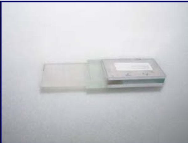
SGP Laminate Bonded to Aluminum
