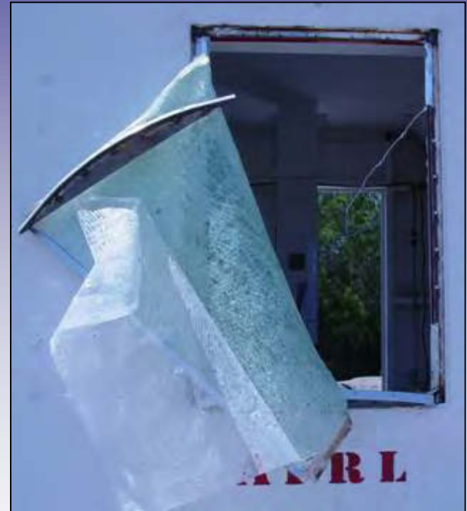
LAMLOK PVB, Bent Glass SUCCESSFUL
