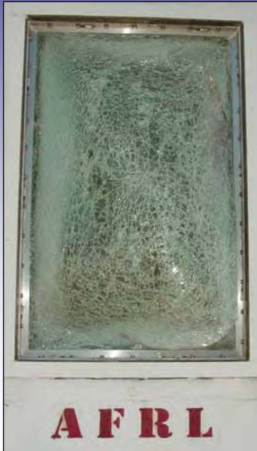
0.180" PVB Clamped Tail SUCCESSFUL
