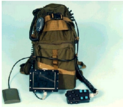
Figure 8. OCU pack with pendant, video display and 8.5db patch antenna.
