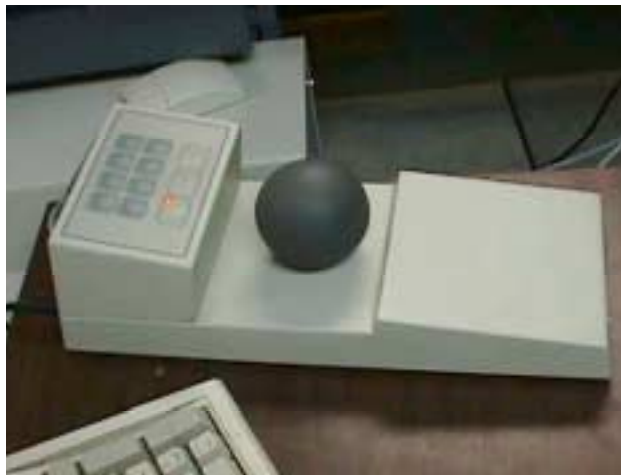
Figure 9: The Space Ball Controller by Force Sensor
