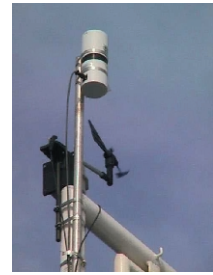
FIGURE 8. The Biospherical Instruments PRR-610 surface irradiator, the NEXUS wind transducer, and the NEXUS magnetic compass are used to measure surface conditions.
