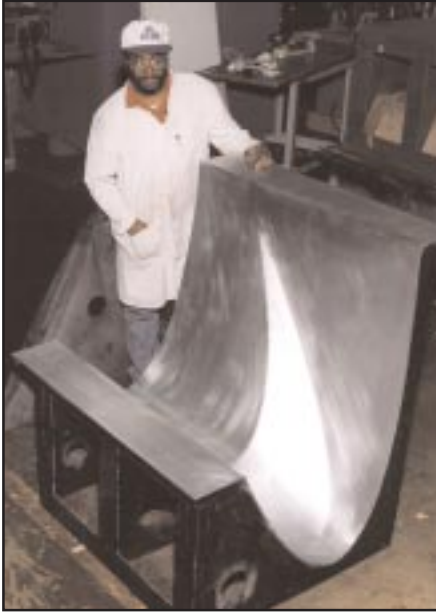
■ The C-17 leading-edge fairing composite tools.
